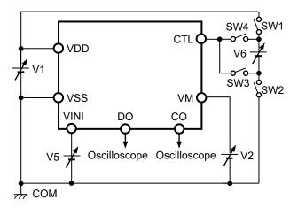
Figure 7 Test Circuit 5
