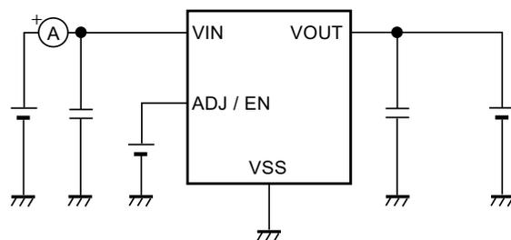
Figure 7 Test Circuit 4
