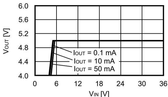
3. Output voltage vs. ADJ / EN pin input voltage (Ta = +25°C)
