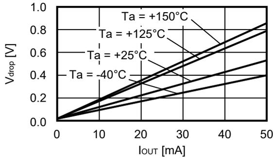
**5. Dropout voltage vs. Junction temperature**
