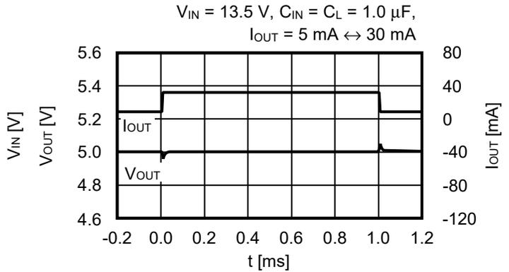
3. Transient response characteristics of ADJ / EN pin (Ta = +25°C)
