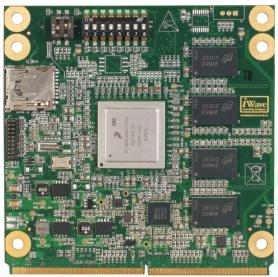
The i.MX6 MXM SOM is based on Freescale's i.MX6 Series Quad/Dual/Solo core processor running at 1GHz.A single ruggedized MXM connector provides the carrier board interface to carry all the I/O signals to and from the MXM module. With 1080p HD decoding & encoding and 2D/3D graphics an enhanced and optimized user experience is achieved.
