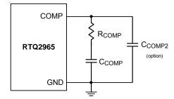
Figure 8. External Compensation Components
