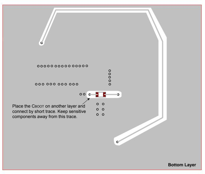
Figure 18. Layout Guide for RTQ2965GQW (Bottom Layer)
