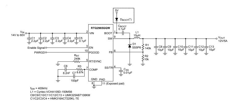
\* : While the input voltage is below 5.5V or duty ratio is higher than 65%, an external bootstrap diode must be added between an external 5V voltage supply and the BOOT pin to enhance the drive capability for the high-side MOSFET. Refer to the Application Information for more details on the external bootstrap diode design.
