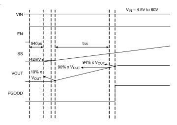
Figure 1 Start-Up Sequence for RTQ2965GQW
