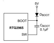
Figure 10. External Bootstrap Diode
