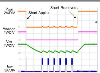
Figure 3. Short-Circuit Protection and Recovery
