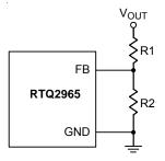
Figure 7. Output Voltage Setting
