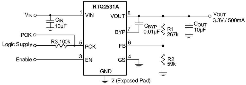
$$V_{OUT} = V_{REF} \times \left( 1 + \frac{R1}{R2} \right) = 0.6V \times \left( 1 + \frac{267k}{59k} \right) = 3.3V$$
