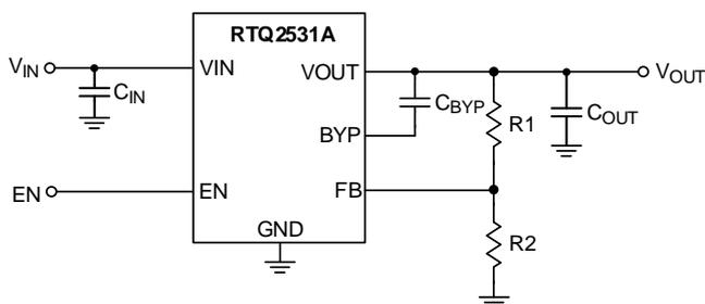
Figure 1. Output Voltage Set by External Resistors
