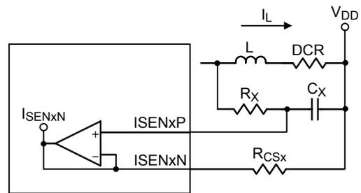
Figure 7. Lossless Inductor Sensing
