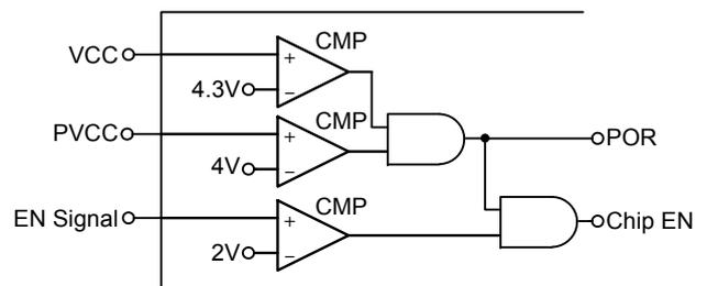
Figure 13. Power Ready (POR) Detection
