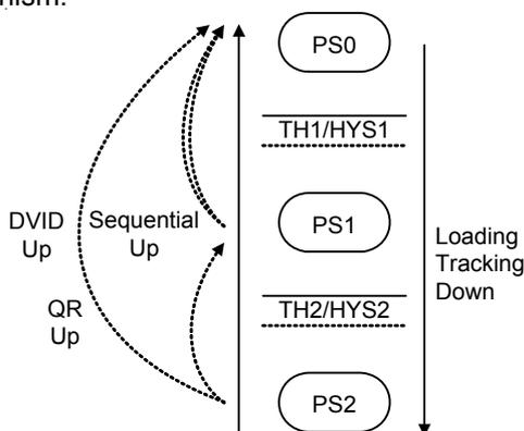
Figure 16. Dynamic Phase Control Mechanism
