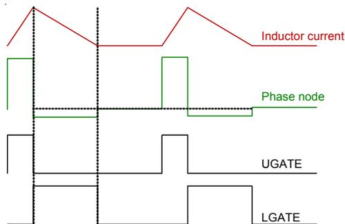
Figure 3. Diode Emulation Mode (DEM) in Steady State
