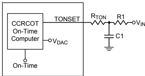
Figure 6. CORE VR : On-Time Setting with RC Filter
