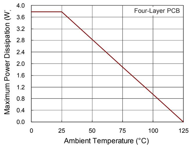
Figure 22. Derating Curve of Maximum Power Dissipation
