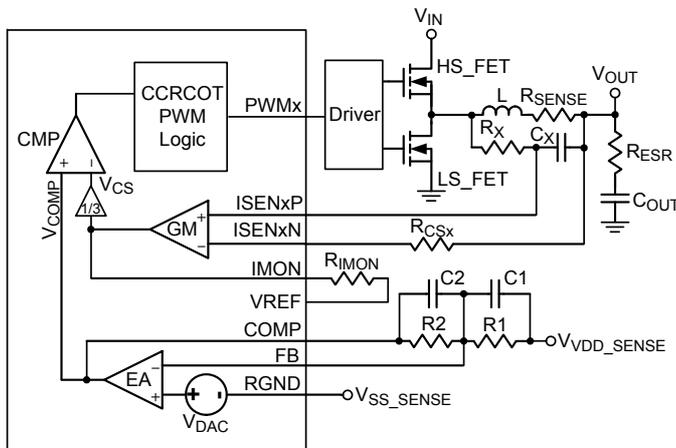
Figure 1. Simplified Schematic for Droop and Remote Sense in CCM
