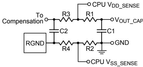
Figure 5. Differential Remote Voltage Sense Connection
