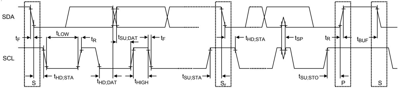
Figure 21. I<sup>2</sup>C Waveform Information
