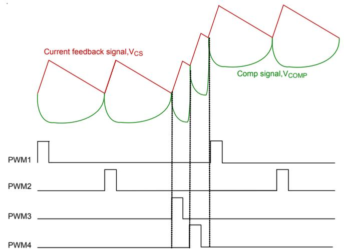
(b). G-NAVP™ Behavior Waveforms in CCM in Load Transient
