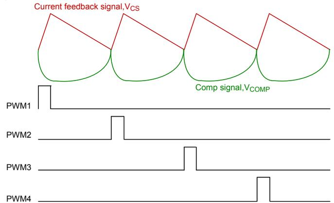
(a). G-NAVP™ Behavior Waveforms in CCM in Steady State
