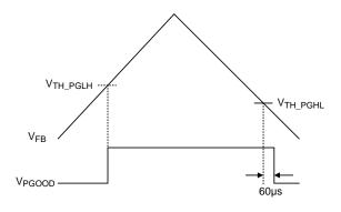
Figure 2. The Logic of PGOOD
