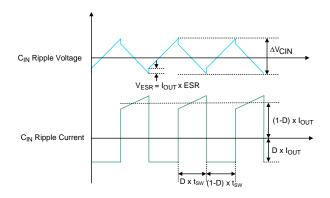
Figure 5. CIN Ripple Voltage and Ripple Current
