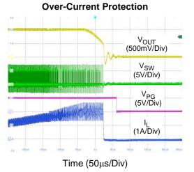
Figure 3. Over-Current Protection
