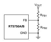
Figure 6. Output Voltage Setting
