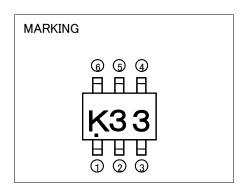
Composite Transistor For high speed switching Silicon N-channel MOSFET
