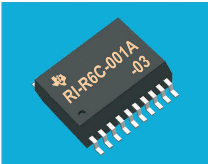
Figure 1-1. S6700 Multi Protocol Transceiver IC (RI-R6C-001A)
