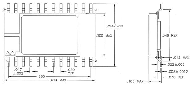
Note: Package and lid are electrically isolated from signal pads.
