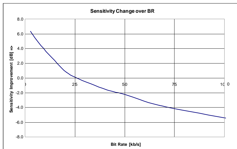
Figure 68: FSK Sensitivity vs. BR
