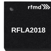
Package: MCM, 16-pin, 8.0 mm x 8.0 mm
