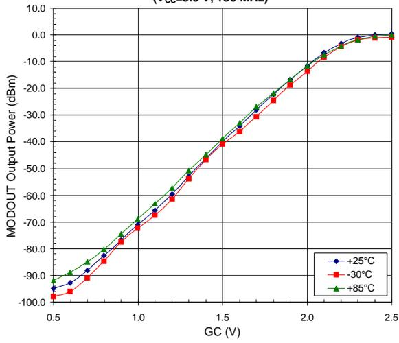
**MODOUT Noise Power versus Gain Control**
