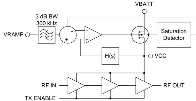
**Figure 2. RF3159 Basic Circuit Diagram**
