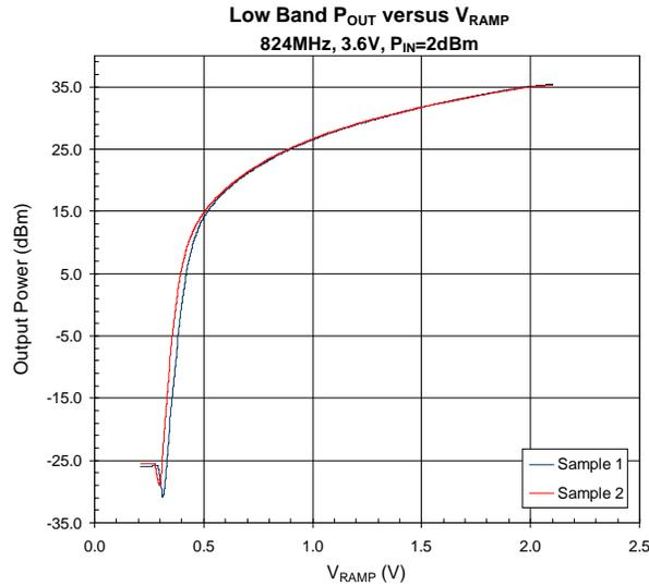
**Figure 3. Graph of Output Power versus  $V_{RAMP}$**
