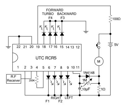
UTC RCT5 output pin (SO) has an inverted phase with UTC RCR5 input (SI). If UTC RCT5 is connected without using a R<sub>F</sub> module, an inverter has to be inserted between this 2 pins.
