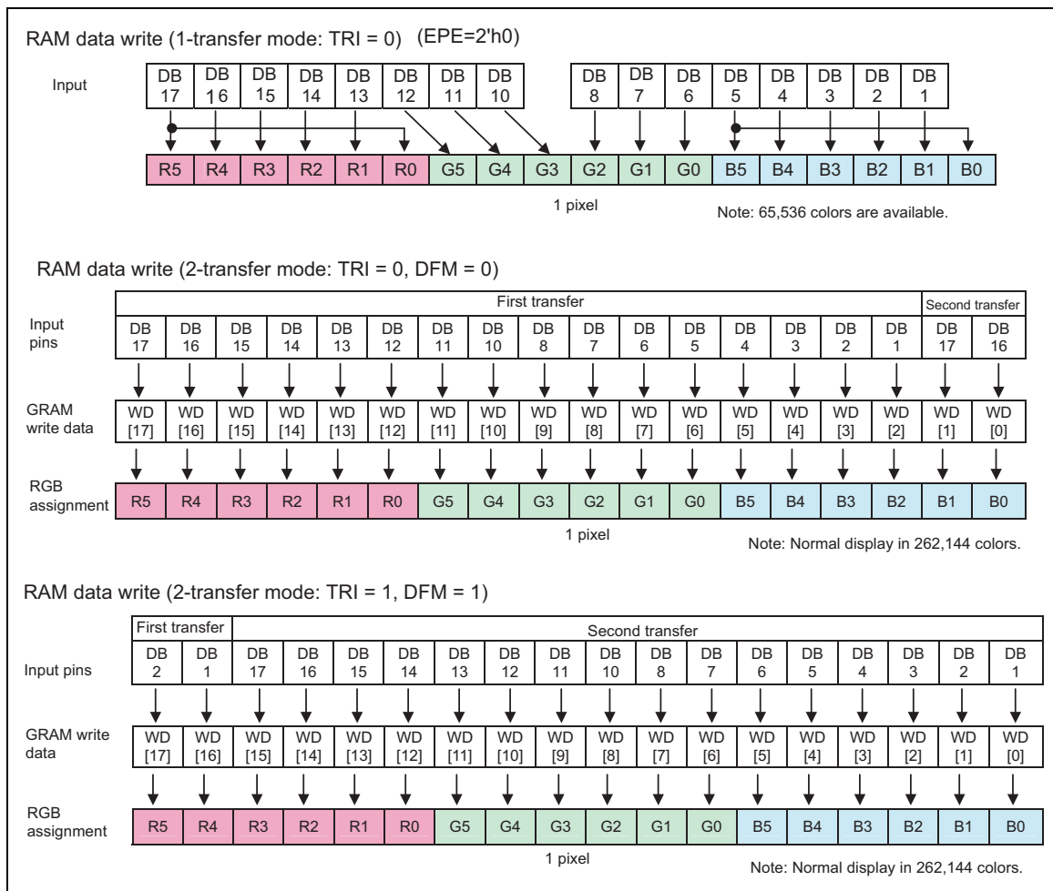
Figure 19 16-bit Interface Data Format (RAM Data Write)
