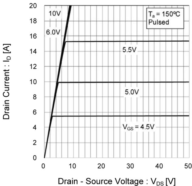
Fig.8  $T_j = 150^\circ\text{C}$  Typical Output Characteristics (II)
