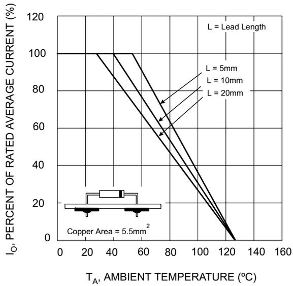
Fig. 1 Current Derating for Various Lead Lengths
