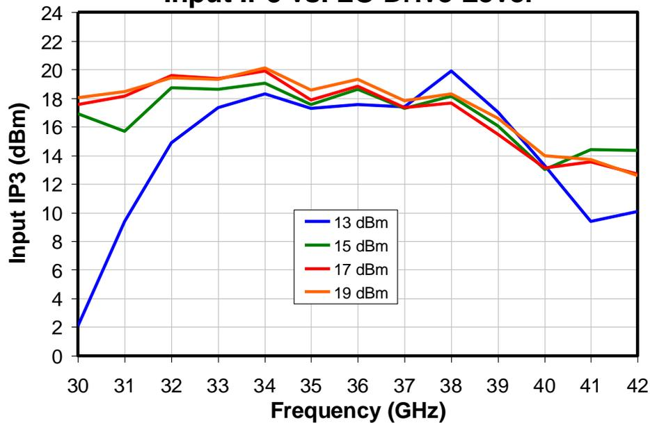
Typical Performance – Data Taken as Upconverter with External IF Hybrid, IF=950 MHz USB
