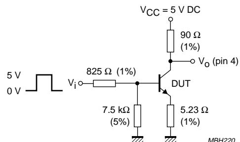
Fig.2 Switching times test circuit.
