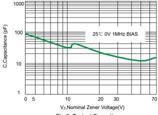
Fig 2. Typical Capacitance
