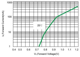
Fig 1.Typical Forward Voltage
