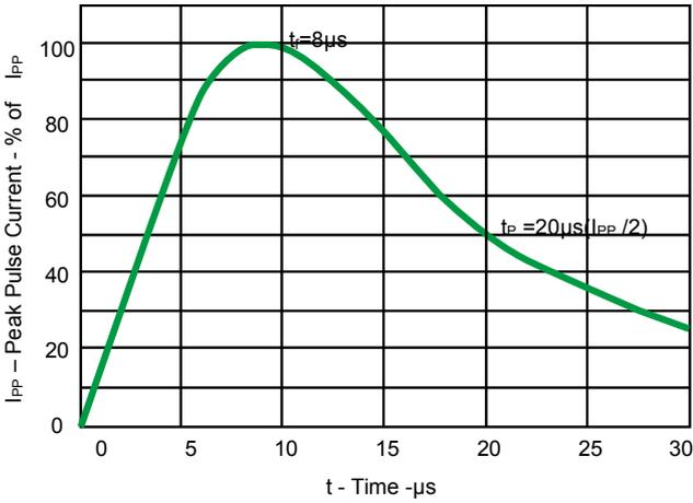
Fig 1. Pulse Waveform
