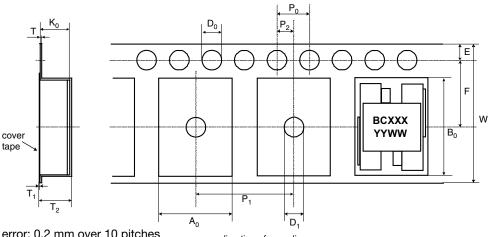
Cumulative pitch error: 0.2 mm over 10 pitches Cumulative tolerance over 10 holes:  $\pm$  0.2 mm
