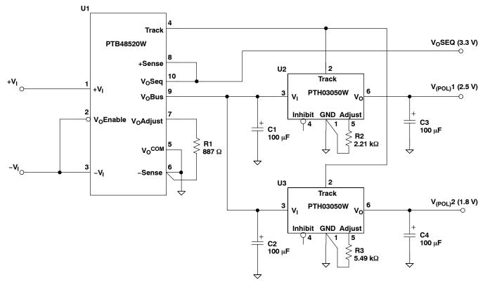
Figure 10. Power-Up Sequencing With Non-Isolated POL Modules
