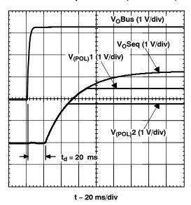
Figure 9. Power-Up Waveforms with POL Modules
