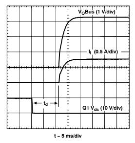
Figure 7. Output Enable Power-Up Characteristic
