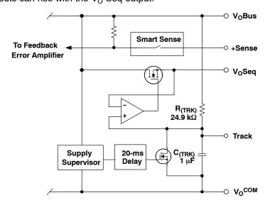
Figure 8. Block Diagram of Auto-Track Features
