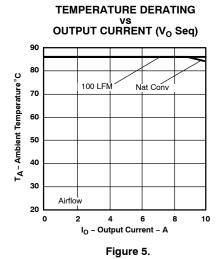
The temperature derating curves represent operating conditions at which internal components are at or below manufacturer's maximum rated operating temperature. See Figure 4 and Figure 5.
