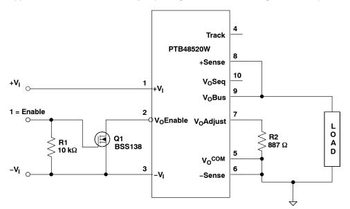
Figure 6. Output Enable Operation
