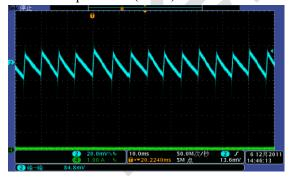
Vin=230Vac, Vout=12V, Iout=1.5A(CC load)
