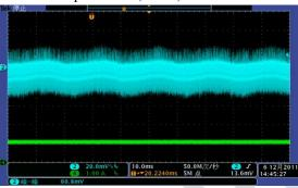
Vin=230Vac, Vout=12V, Iout=0A(CC load)
