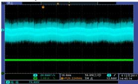
Vin=230Vac, Vout=12V, Iout=0.5A(CC load)
