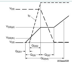
Fig. 13. Gate charge waveform definitions
