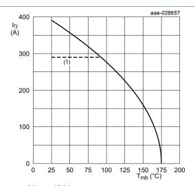
$V_{GS} \ge 10 \text{ V}$  (1) 290A continuous current has been successfully demonstrated during application tests. Practically the current will be limited by PCB, thermal design and operating temperature.
