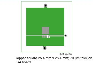
Fig. 5. PCB layout for thermal resistance from junction to ambient
