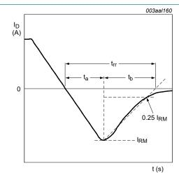
Fig. 16. Reverse recovery timing definition
