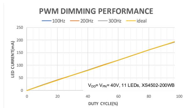
Figure 12. Current accuracy vs PWM dimming
