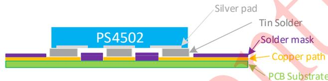
Figure 15. Cross section of PS4502 on PCB.
