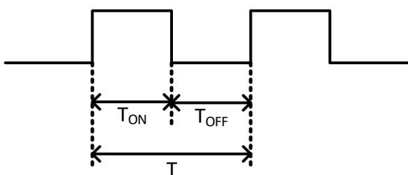
Figure 11. PWM dimming signal
