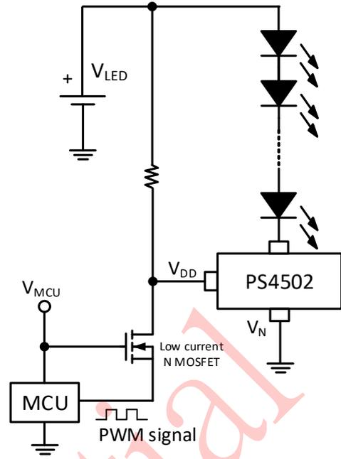
Figure 14. PWM dimming by external MOSFET
