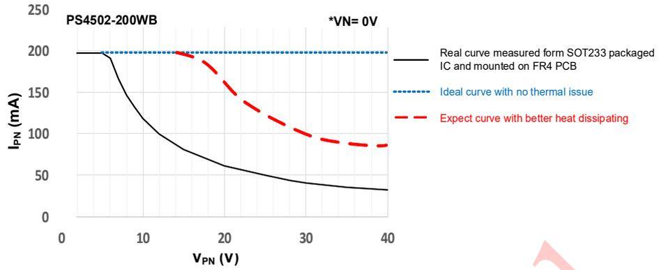
Figure 5. Load regulation, I<sub>PN</sub> vs V<sub>PN</sub>
