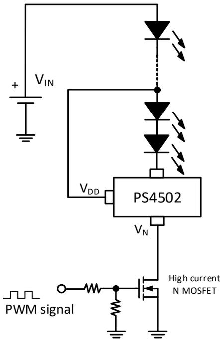
Figure 13. Simplified dimming circuit.
