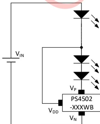
Figure 1. Single channel LED driver
