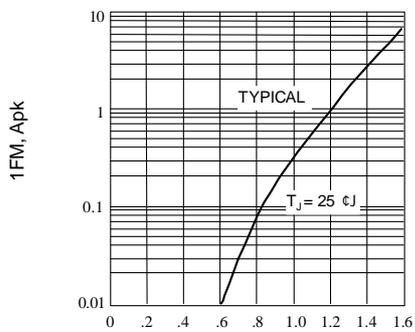
Fig. 2-FORWARD CHARACTERISTICS
