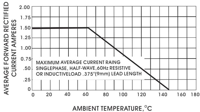
Fig.3-FORWARD DERATING CURVE
