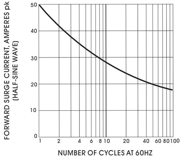
Fig.2-MAXIMUM OVERLOAD SURGE-CURRENT
