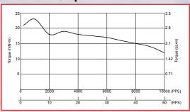
Excitation Mode: Full-step Voltage: 24VDC Current: 0.78A
