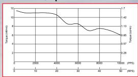
Excitation Mode: Full-step Voltage: 24VDC Current: 0.6A
