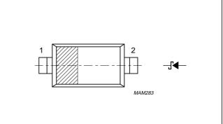
Marking code: E2. The marking bar indicates the cathode.
