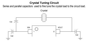
CST – Series Capacitor, used to lower circuit load to match crystal load. Raises frequency offset. This can be eliminated by using a crystal with a Cload of equal or greater value than the oscillator CPT – Parallel Capacitors, Used to raise the circuit load to match the crystal load. Lowers frequency offset.
