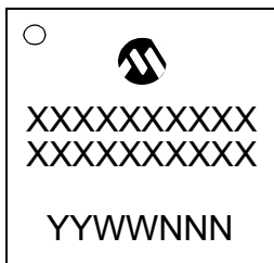
64-Lead QFN (9x9x0.9mm)
