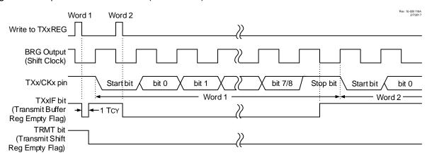
Figure 31-4. Asynchronous Transmission (Back-to-Back)
