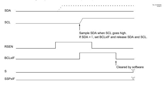
If SCL goes from high-to-low before the BRG times out and SDA has not already been asserted, a bus collision occurs. In this case, another host is attempting to transmit a data '1' during the Repeated Start condition (see Figure 30-38).
