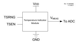
The output of the circuit is measured using the internal Analog-to-Digital Converter. A channel is reserved for the temperature circuit output. Refer to the "ADC - Analog-to-Digital Converter with Computation Module" chapter for more details.
