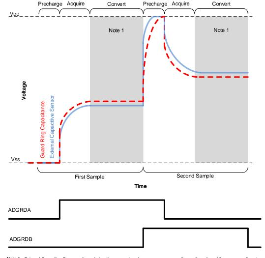
Note 1: External Capacitive Sensor voltage during the conversion phase may vary as per the configuration of the corresponding pin.
