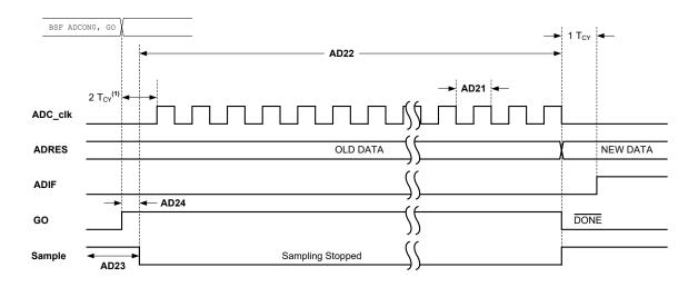
1. If the ADC clock source is selected as ADCRC, a time of  $T_{CY}$  is added before the ADC clock starts. This allows the SLEEP instruction to be executed.
