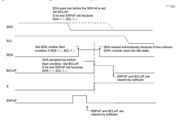
The Start condition begins with the SDA and SCL pins deasserted. When the SDA pin is sampled high, the Baud Rate Generator is loaded and counts down. If the SCL pin is sampled low while SDA is high, a bus collision occurs because it is assumed that another host is attempting to drive a data '1' during the Start condition.
