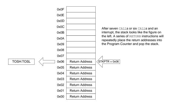
Figure 9-19. Accessing the Stack Example 4
