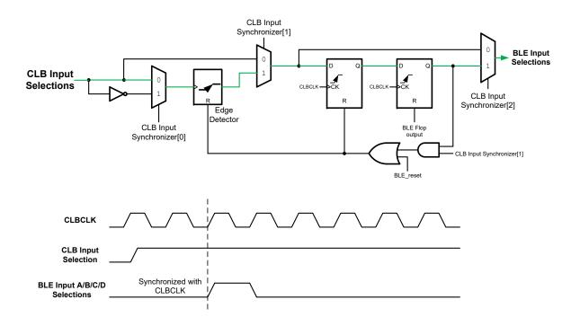
Figure 29-9. Edge Detector Operation when CLB Input Synchronizer[2:0] = '111'
