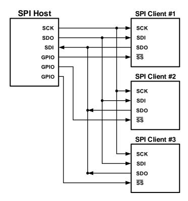
Transmissions involve two shift registers, eight bits in size: One in the host and one in the client. Data are shifted out one bit at a time, with the Most Significant bit (MSb) shifted out first. At the same time, a new Least Significant bit (LSb) is shifted into the same register.
