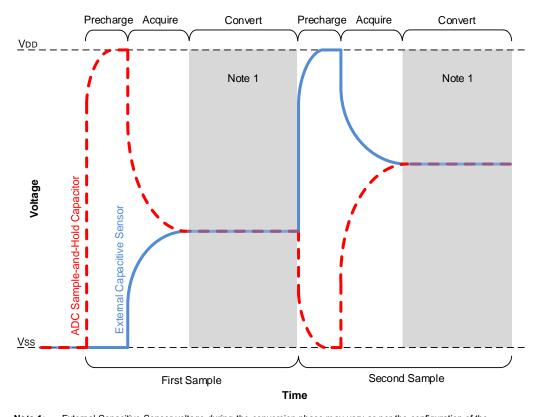
**Note 1:** External Capacitive Sensor voltage during the conversion phase may vary as per the configuration of the corresponding pin.
