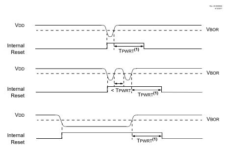
**Note:**  $T_{PWRT}$  delay when the PWRTS bits are enabled ( $\overline{PWRTS}$  != 00).
