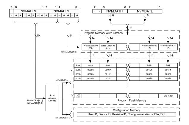
Figure 15-5. Program Flash Memory Write Sequence
