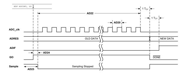
Figure 41-10. ADC Conversion Timing (ADC Clock from ADCRC)
