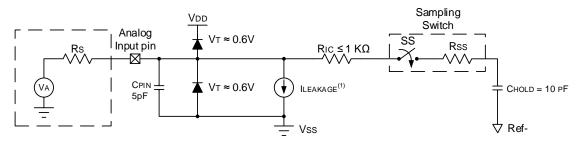
Legend: CPIN = Input Capacitance ILEAKAGE = Leakage Current at the pin due to various junctions = Interconnect Resistance Sampling Rs = Source Impedance Switch Rss VA = Analog Voltage  $(K\Omega)$ = Diode Forward Voltage Vт = Sampling Switch = Resistance of the Sampling Switch Rss 3 4 5 6 = Sample/Hold Capacitance CHOLD  $V_{DD}$ (V)
