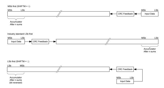
When the SHIFTM bit is not set, data will be shifted into the CRC, MSb first and the result will be big-endian. When the SHIFTM bit is set, data will be shifted into the accumulator in the reversed order (LSb first) and the result will be little-endian. The CRC module can be seeded with an initial value by setting the CRCOUT registers to the appropriate value before beginning the CRC process.
