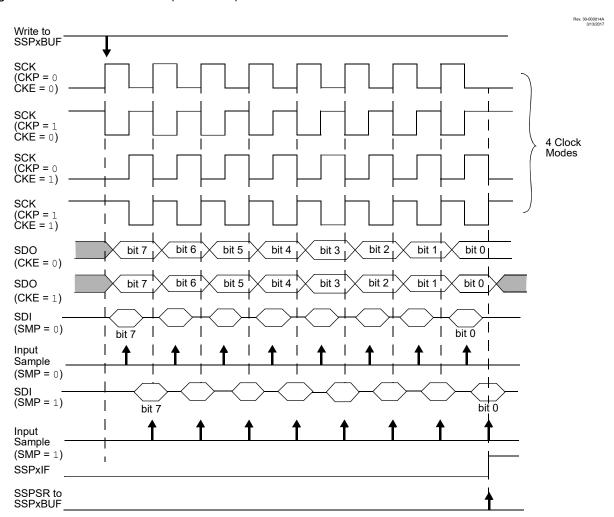
Figure 30-4. SPI Mode Waveform (Host Mode)
