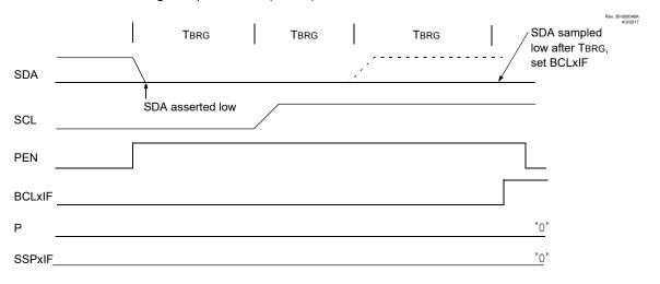
Figure 30-40. Bus Collision During a Stop Condition (Case 2)
