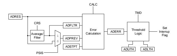
The operation of the ADC computational features is controlled by the MD bits.
