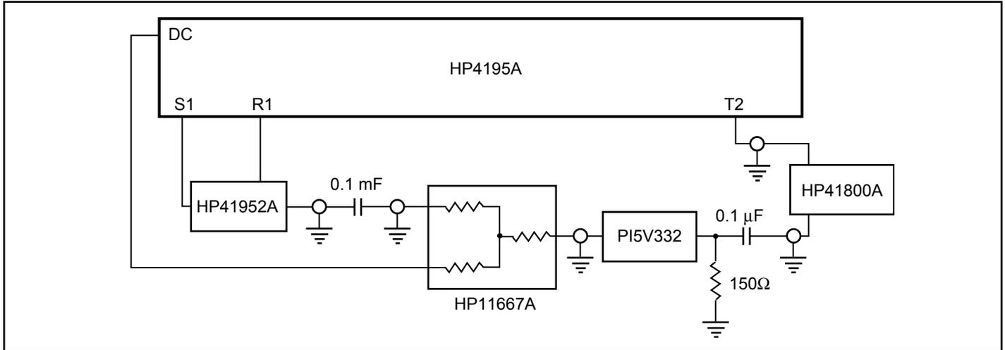
Figure 1. Differential Gain/Phase
