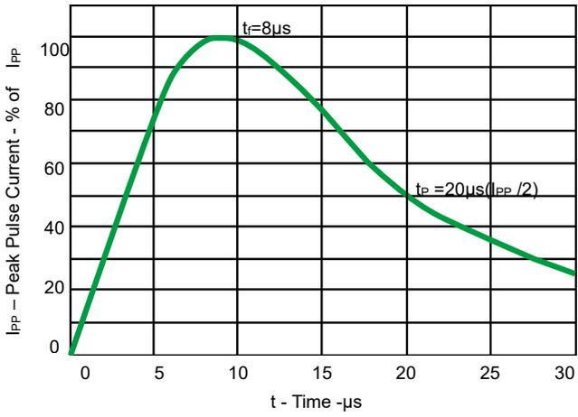
Fig 1. Pulse Waveform
