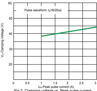
Fig 3. Clamping voltage vs. Peak pulse current
