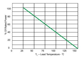
Fig 2.Power Derating Curve
