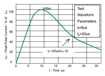
Fig 1.Pulse Waveform
