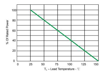
Fig 2.Power Derating Curve
