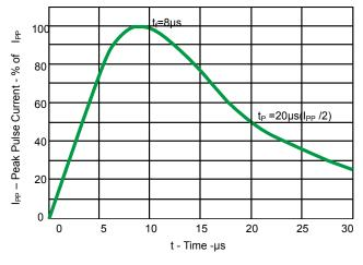
Fig 1.Pulse Waveform
