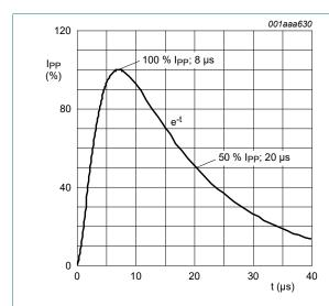
Fig. 2. 8/20 µs pulse waveform according to IEC 61000-4-5 and IEC 61643-321
