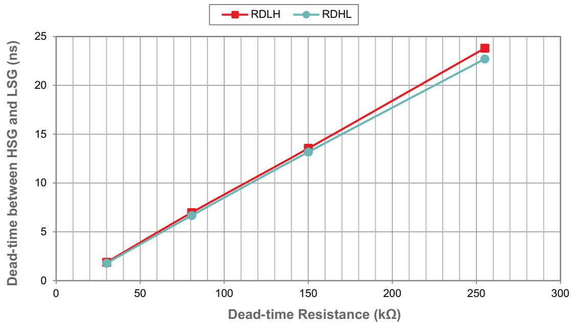
Figure 7 ■ Dead-time between HSG and LSG (ns)
