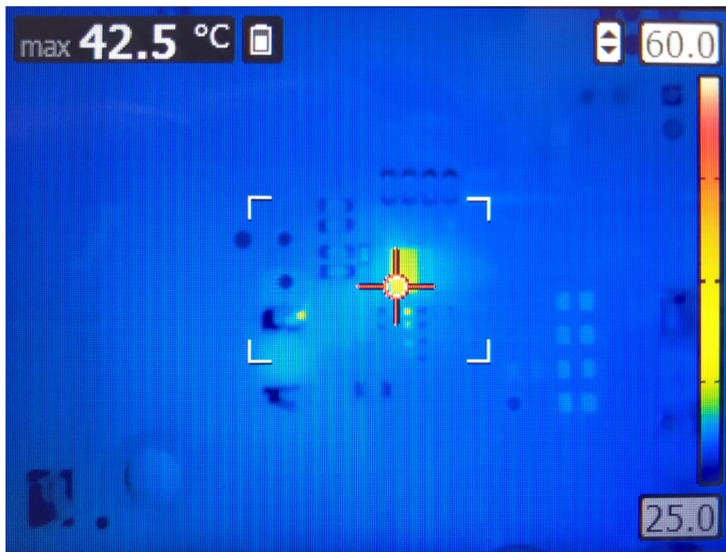
Figure 31. PE23108 Thermal Performance
