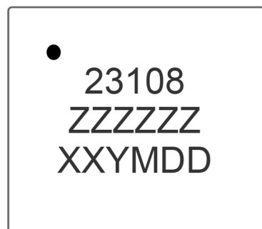
Figure 51. 3.445 mm x 2.095 mm WLCSP Package Marking Specifications
