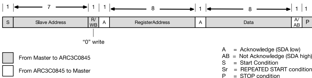
Figure 42. "Write" Data Transfer Format in Standard, Fast, Fast-Plus Modes
