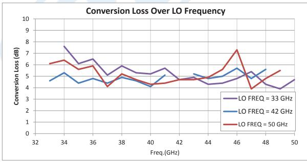
Click the following link (or enter part number in "SEARCH" on website) to obtain additional part information including price, inventory and certifications: Waveguide Mixer Down Converter WR-22 From 33 GHz to 50 GHz, IF From DC to 18 GHz And LO Power of +13 dBm, UG-383/U Flange, Q Band PE12D1004
