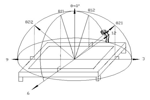
Note 12-2: CR = Luminance when Testing point is White Luminance when Testing point is Black
