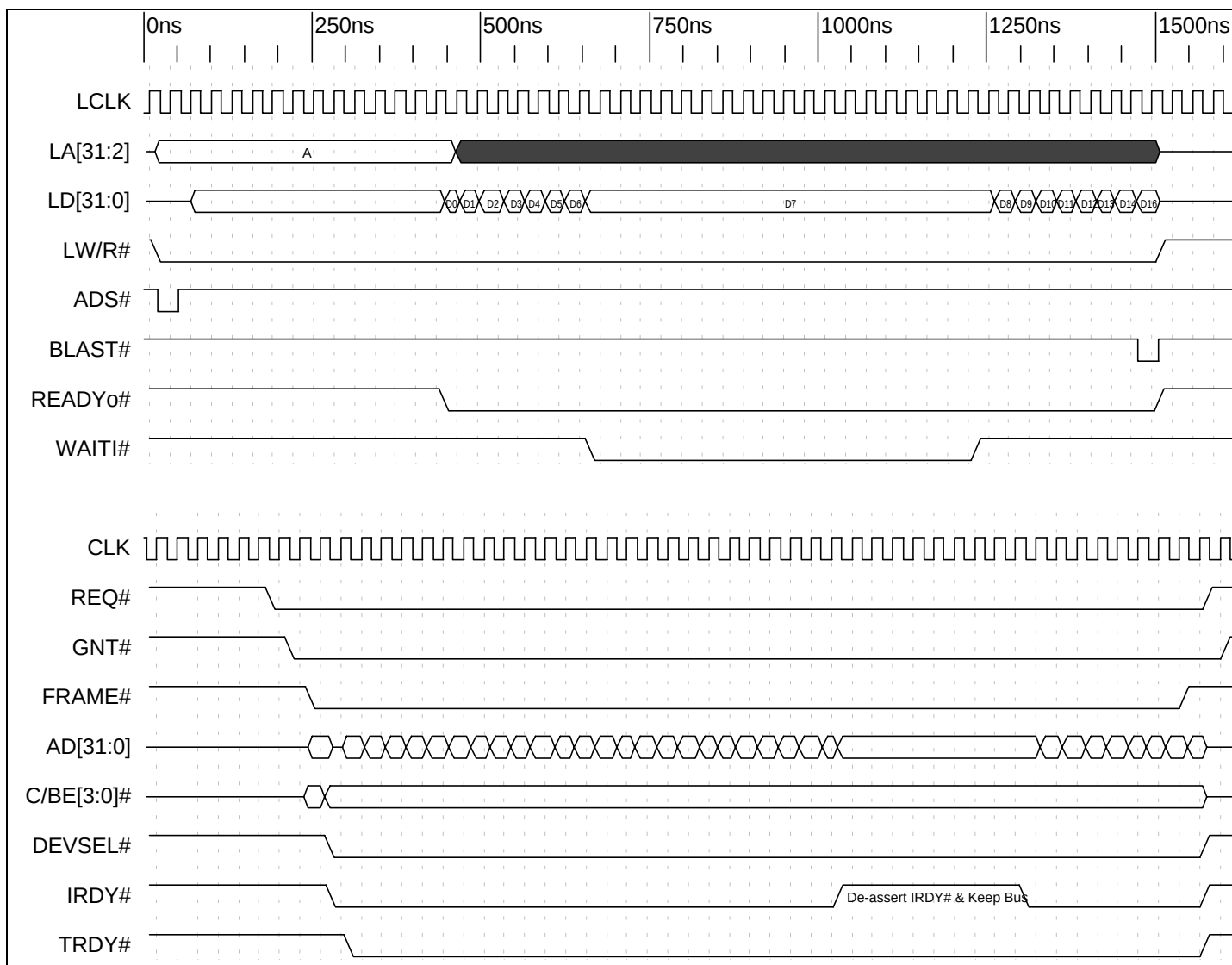
Timing Diagram 8-42. (C Mode) PCI 9080 Direct Master Memory Read—Keep Bus
