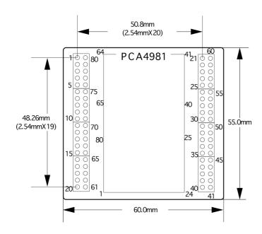
st Pins and other parts needed to connect the standard pitch converter are not included with the product.
