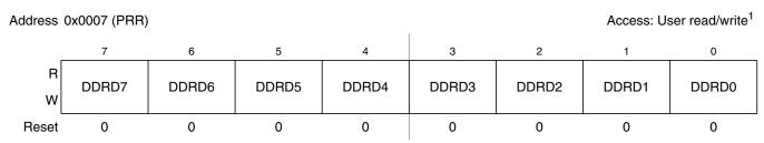
Figure 2-8. Port D Data Direction Register (DDRD)
