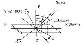
Light (when transmitted )  $Y(\varnothing=0^{\circ})$   $(\theta=90^{\circ})$
