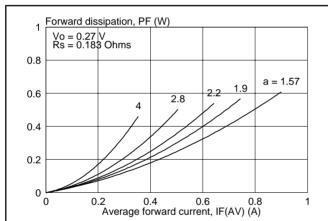
Fig.3. Maximum forward dissipation  $P_F = f(I_{F(AV)})$  per diode; sinusoidal current waveform where a = f form factor  $= I_{F(RMS)} / I_{F(AV)}$ .
