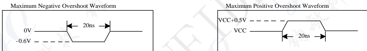
Figure 5-1 Maximum Overshoot Waveform
