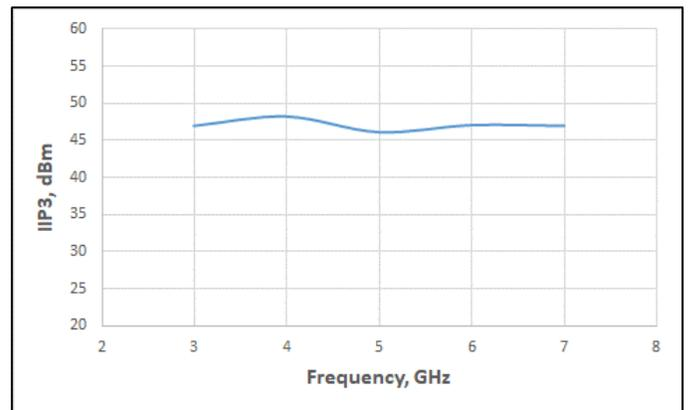
Figure 7 – In-Band IIP3 vs Frequency
