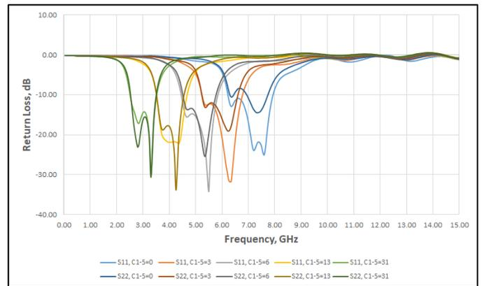
Figure 4 – Overlaid S11 and S22 Return Loss
