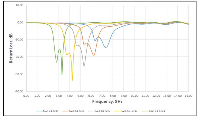
Figure 3 – Output Return Loss vs Grouped Tuning Settings
