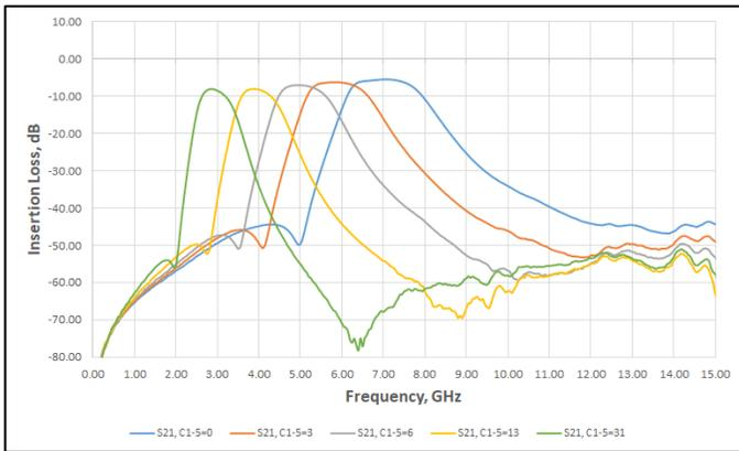
Figure 1 – Insertion Loss vs Grouped Tuning Settings
